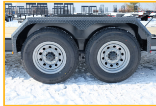
Steel Mod Wheels with Radial Tires
