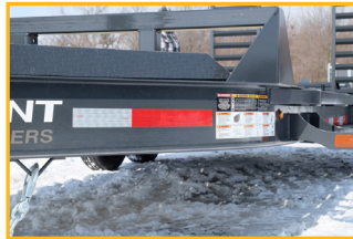
Heavy-Duty 8" Formed I-Beam Frame
